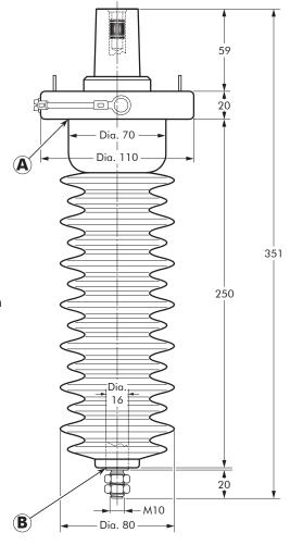
6/10 (12) kV 6.35/11 (12) kV 8.7/15 (17.5) kV 12/20 (24) kV 12.7/22 (24) kV
