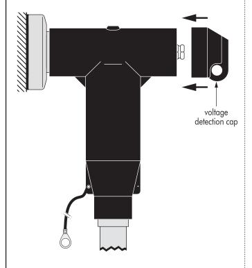
Clean inner surface of voltage detection cap (do not lubricate) and place on the connector. Push down hard until cap "snaps" into place.
