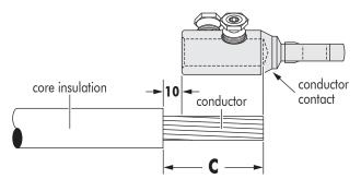
B. Remove the core insulation from the conductor for a distance **« C »** mm (**C** = depth of contact bore + **10** mm).
