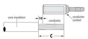
A. Remove the core insulation from the conductor for a distance **« C »** mm
